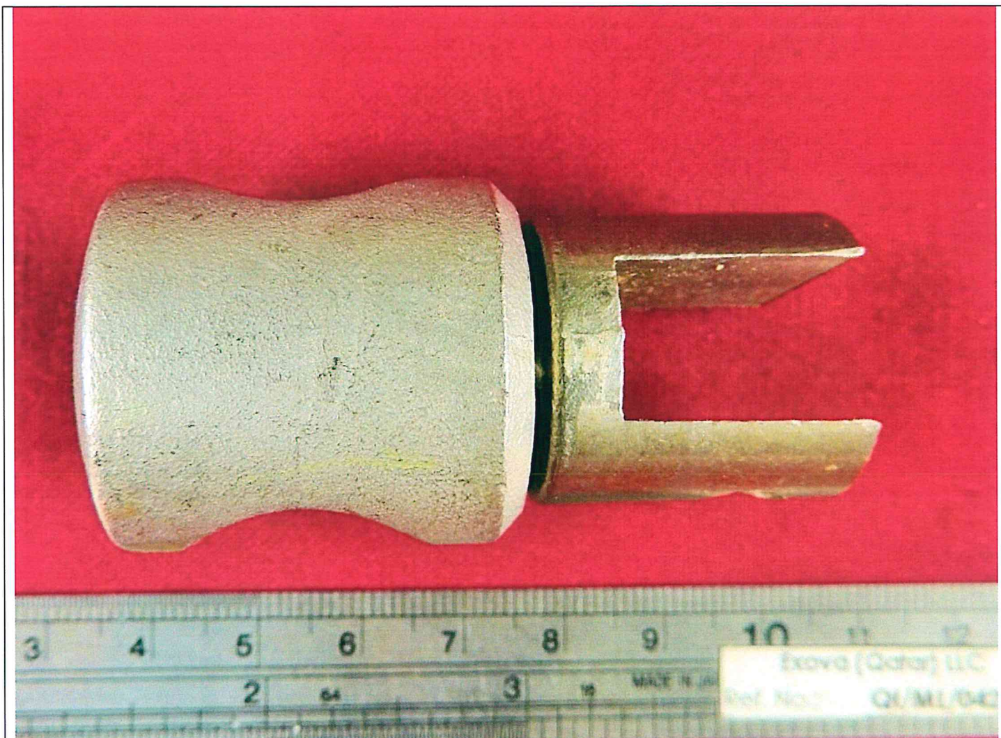
Figure 1: Photograph showing as-received condition of Pipe-Glass Connector sample for PMI testing.
