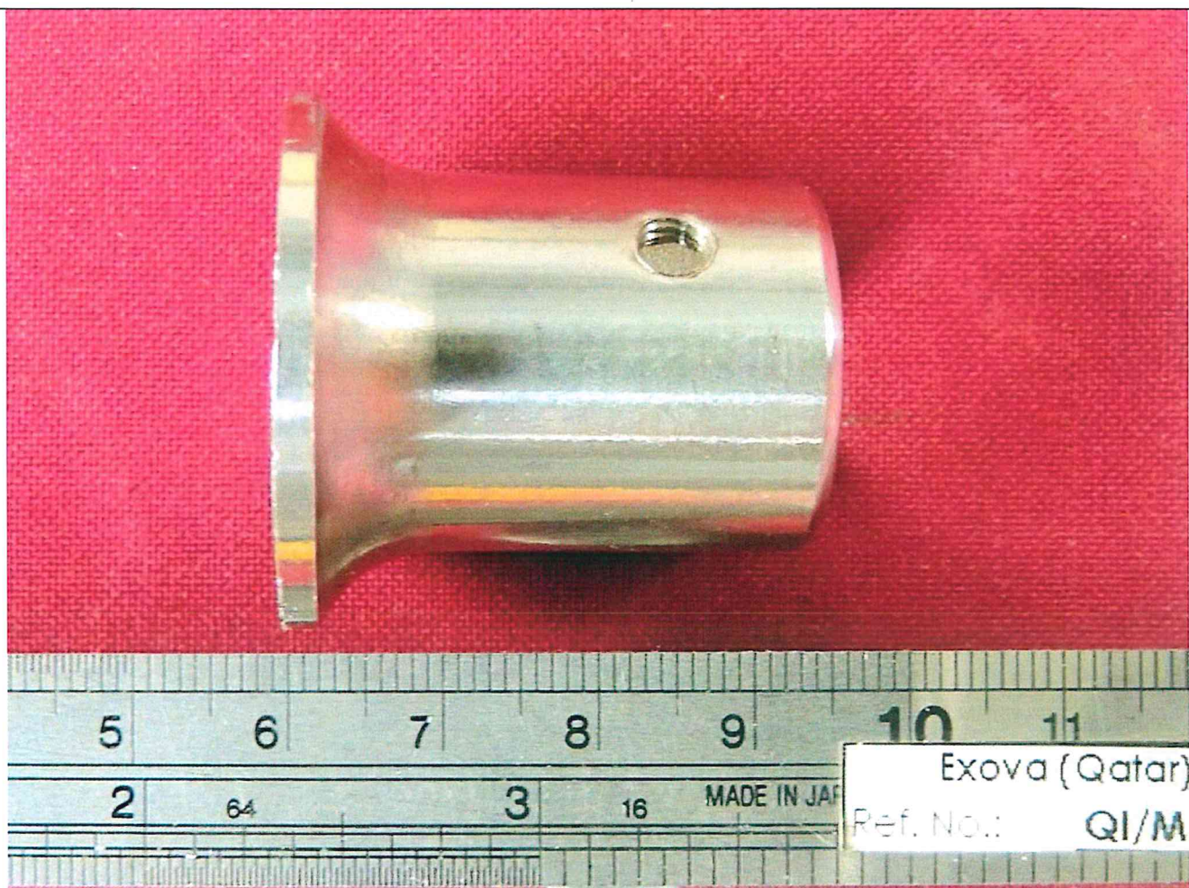
Figure 1: Photograph showing as-received condition of Pipe-Valve Connector for PMI testing.
